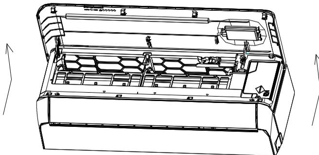
2. Take off the cover of USB Wi-Fi, follow the arrow and insert the USB Wi-Fi module into the reserved USB slot on the frame.
