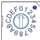
The rotating coded switch S3(0-F) on the main control board of hydraulic module is used for set the modbus address.
