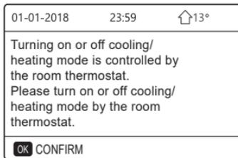
② DUAL ROOM THERMOSTAT is set YES(see "ROOM THERMOSTAT SETTING" in "Installation and owner's manual (Optimus Pro split indoor unit)").The room thermostat for fan coil is turned off ,the room thermostat for the floor heating is turned on,and the unit is running, but the display is OFF. The following page is displayed:
