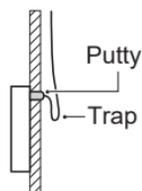
Avoid the water enter into the wired remote controller, use trap and putty to seal the connectors of wires during wiring installation.
